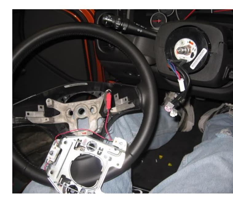
12) Remove back plastic cover from steering wheel Use 3mm hex driver and remove both bolts:
