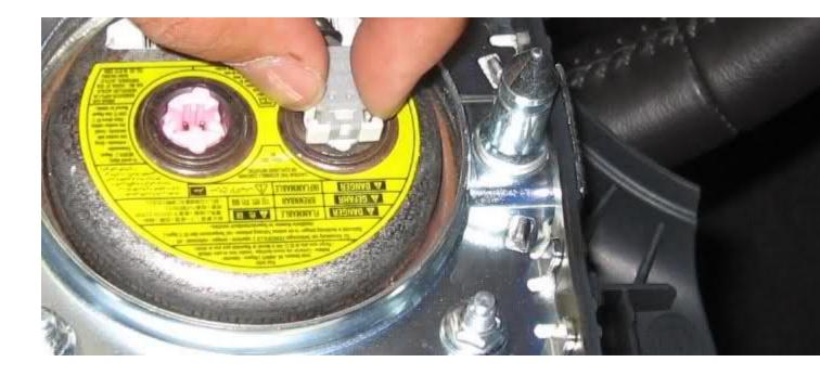
Both wiring harnesses removed; Airbag placed somewhere safe, out of the way:
