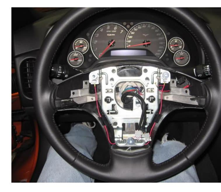
7) Remove Horn electrical frame Unscrew 3 bolts using 4mm hex driver and suitable wrench; bolts remain attached to the frame
