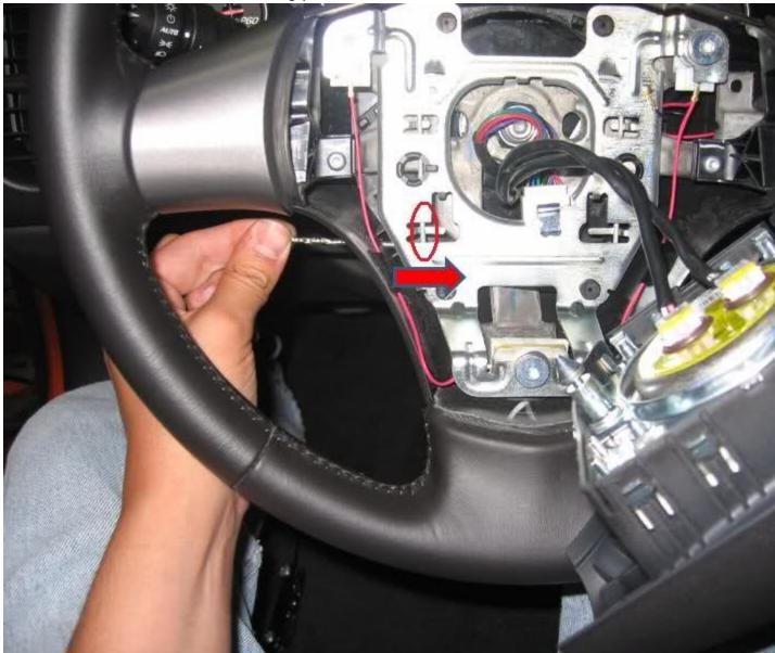
Tool inserted and left side retainer being pushed inward:
