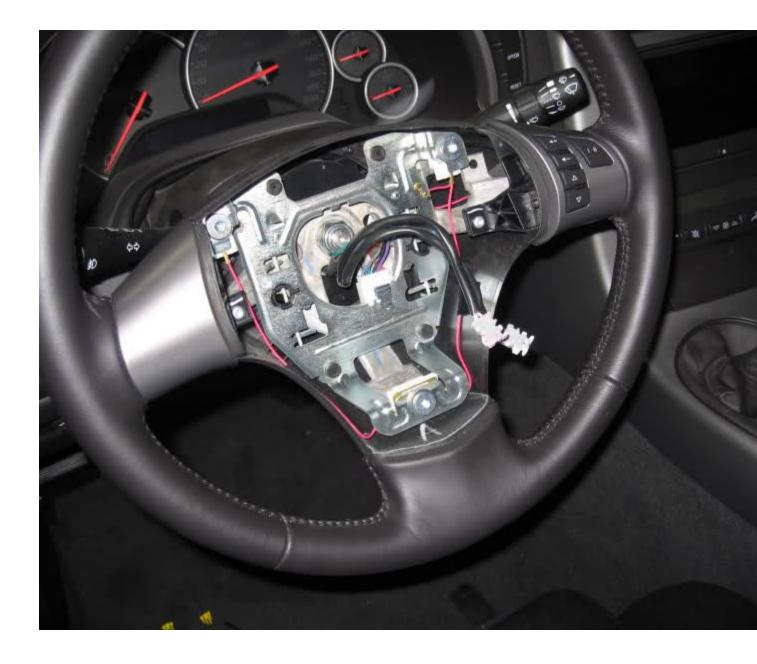
5) Unclip white wiring harness Push up with your finger to unclip Unclipped:
