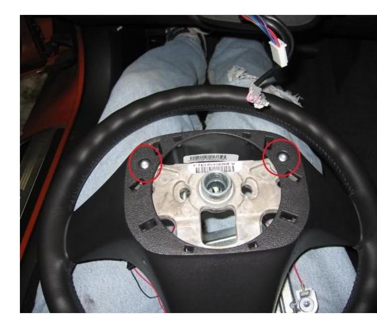
With bolts remove, the back plastic cover comes off, the horn frame comes off, and the steering wheel is loose:
