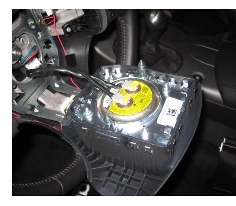
[Side spoke cover replacement, follow step 3; steering wheel replacement, go to step 4] 3a) Remove side covers:
