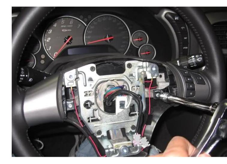
3b) Flip cover over and disconnect electrical connector as needed. Electrical connector:
