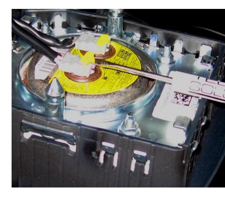
Remove airbag wiring harness by pressing both plastic clips inward with fingers:
