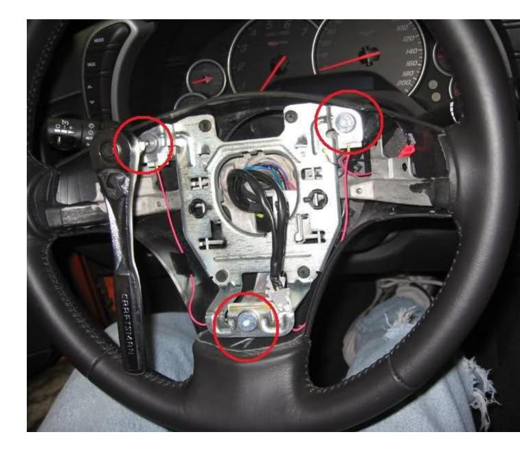
Pull connector out from under metal piece and move frame on top of steering hub:
