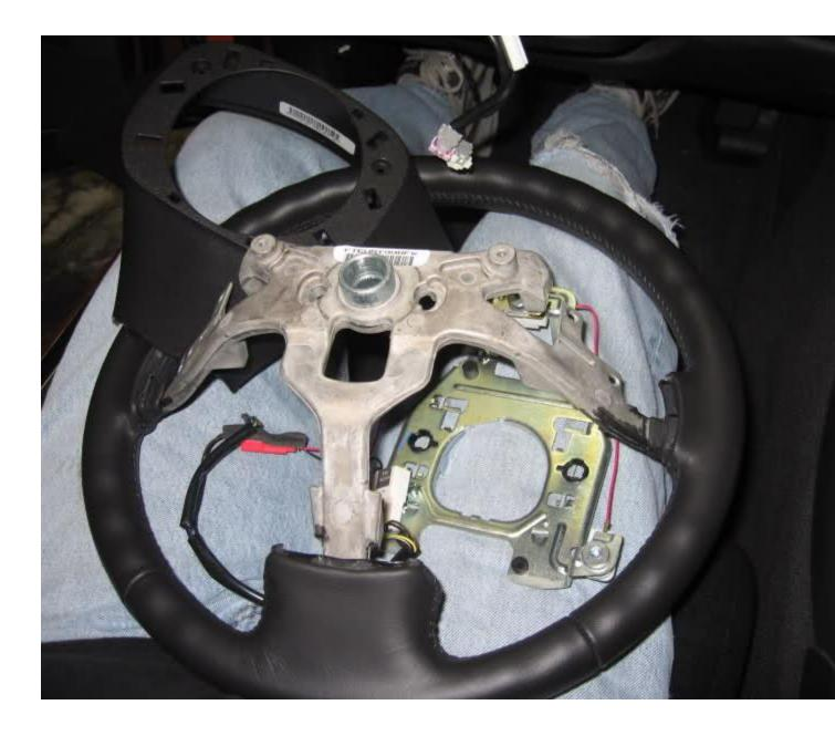
13) That's it... to reinstall, reverse the steps above with your new steering wheel!Torque spec for center nut: **27 lb-ft**All other bolts: Tighten until firm as everything else is plastic against metal.
