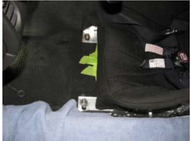
Seat rails fastened to Stud Extenders
