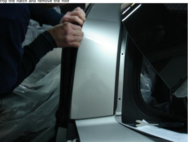
pull the front weatherstrip on the halo by pulling on one side and roll it out down to the plugs/ends on each side. You can leave the weatherstrip attached at the ends and not remove it completely from the vehicle.
