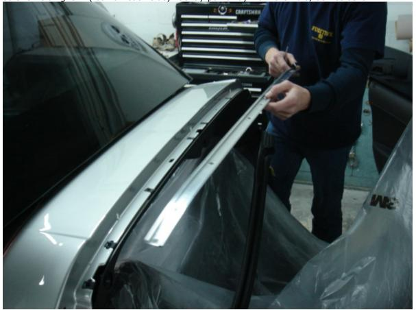
Remove the 4 torx screws from the weatherstrip track on each side. The weatherstrip track on the sides came with my new halo so I didn't pull them off or separate them from the original halo.
