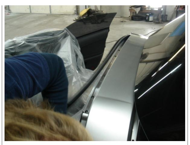
pull the plastic interior trim inside the vehicle underneath the halo. This is attached by four pop in/out clips on each corner. The clips are tight, wiggle them until they pop out or cut the heads off and go buy new when you reinstall. An interior removal tool would help in this area. The interior trim piece is still held together by clips, just pull gently and it will pop out.
