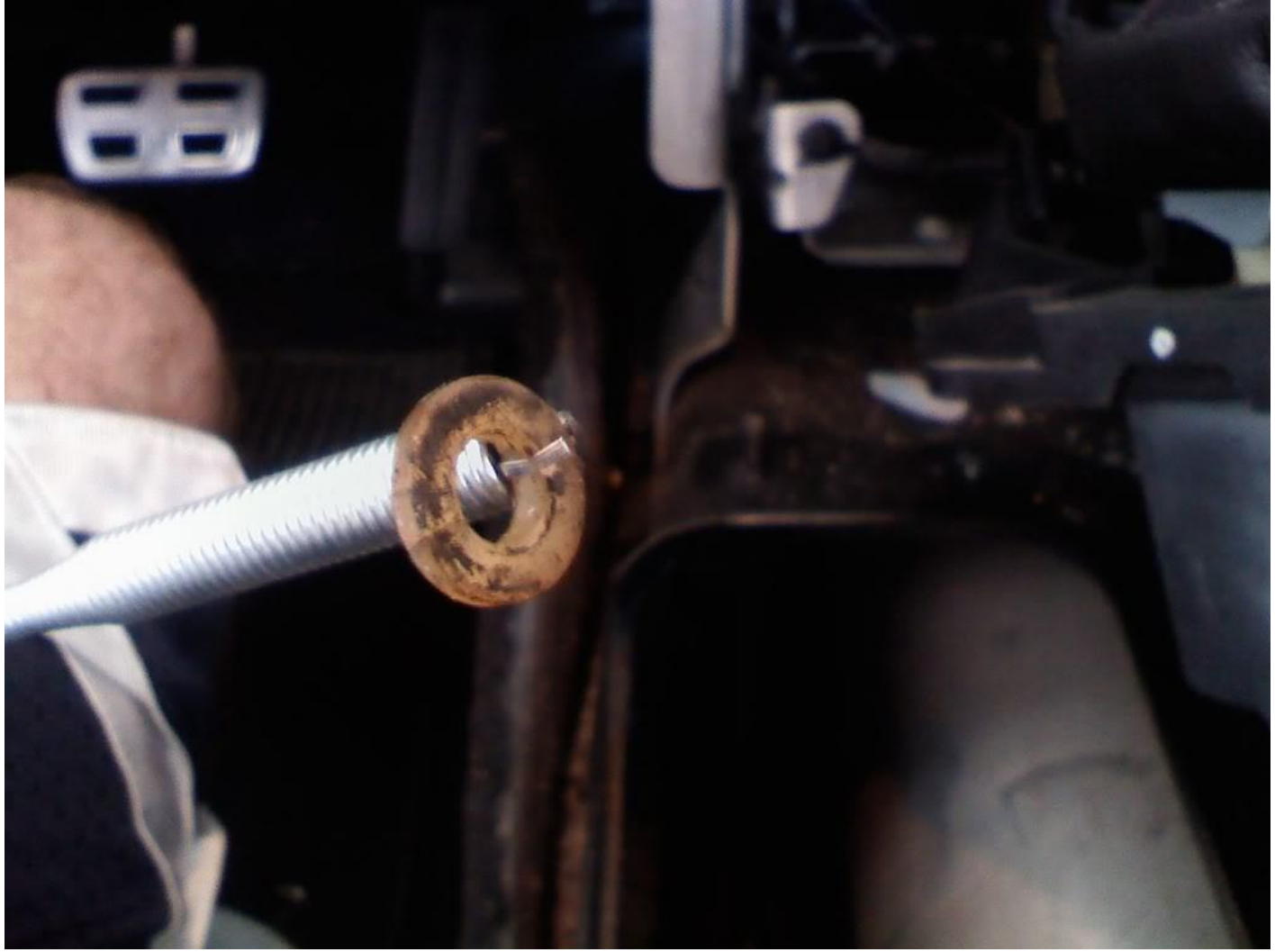
The bushing was dry rotted and cracked
