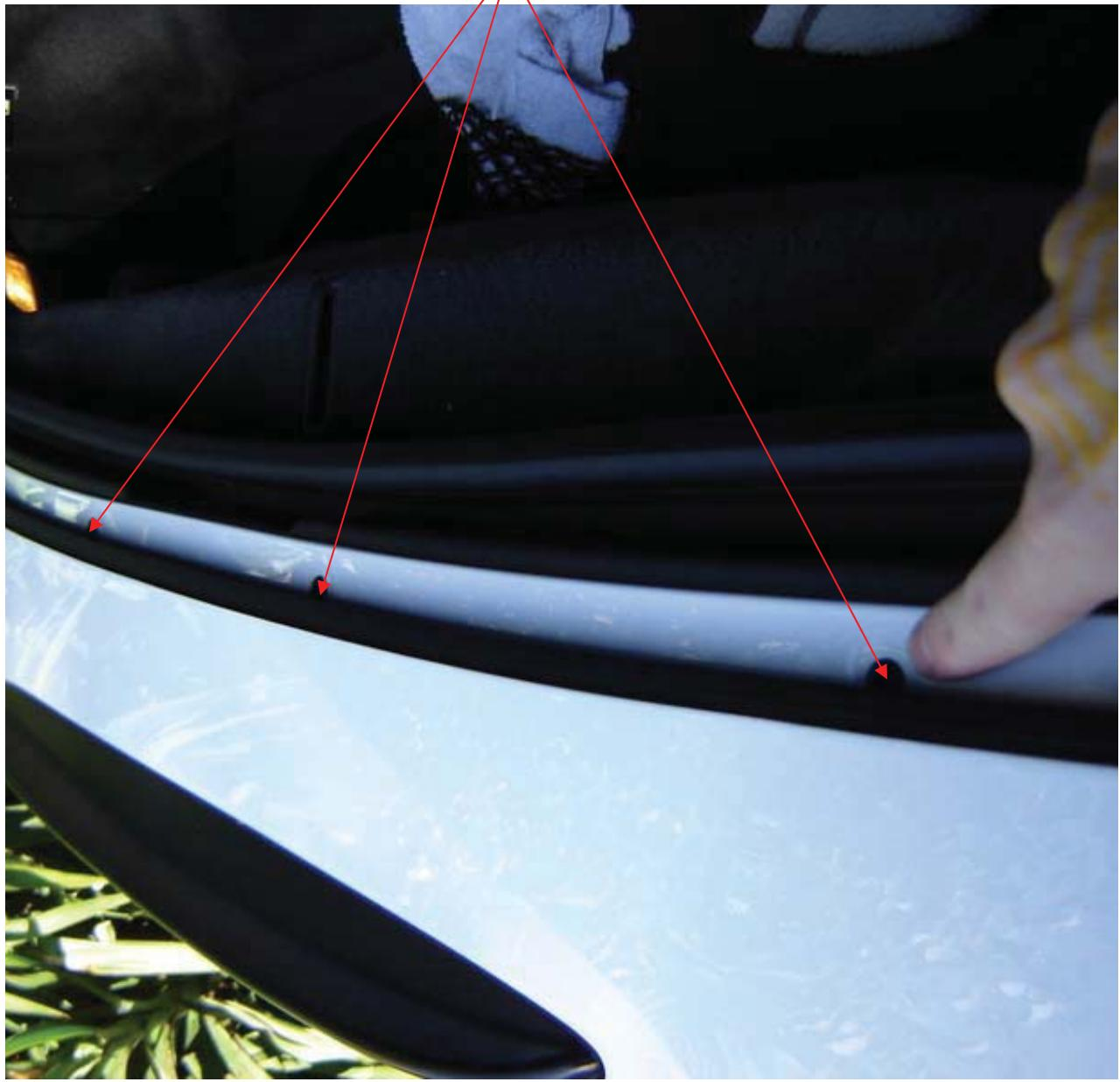
With a T15 torx, remove the 6 torx screws across the inside of the top bumper. You will need to pop the hatch/trunk to do perform this step. Don't worry, the bumper wont fall as it rests on a lip and you have to lift it off the lip to remove it.
