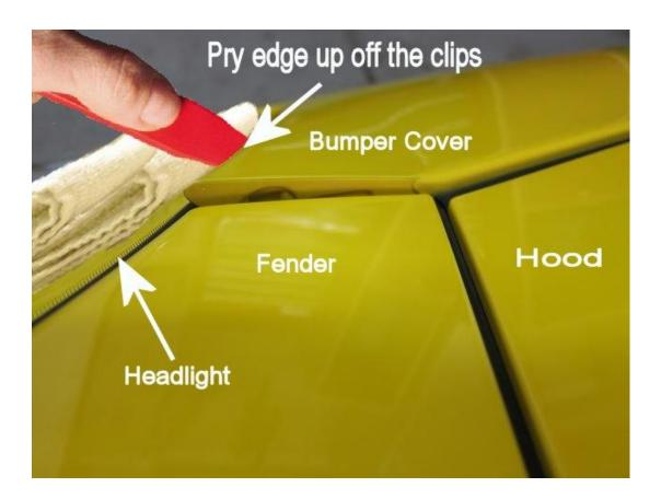
2) Once both sides are popped up from the clips, undo the (4) 9/32" (7mm) bolts that are located on the top portion of the bumper cover. Put masking tape on top of bumper directly under the open hood.
