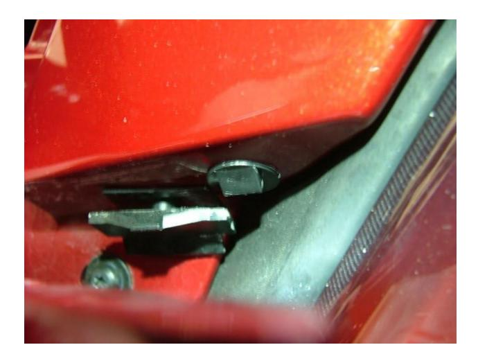
Note: Removing the old clip/locator and inserting new ones can be done without lifting the front bumper cover off the retaining studs, but you will have more room to maneuver if you do slide the bumper cover off the retaining studs.
