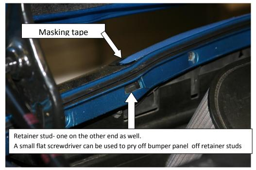
4) Once the front bumper cover is off the retaining studs, then grab under the edge and pull it up out of the way. This will assure you have enough room to remove the old clip and locator.
