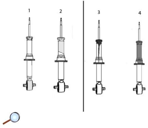
**Do Not Replace coil-over shock absorbers** displaying condition 1 or 2 levels of seepage.
