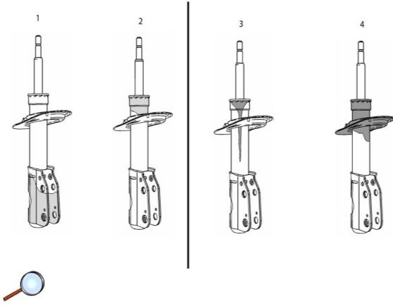
**Do Not Replace Struts** displaying condition 1 or 2 levels of seepage.
