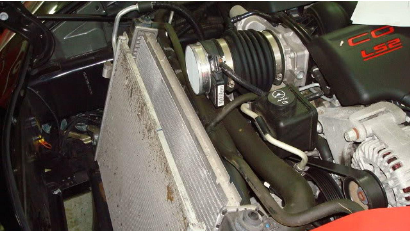
Figure 13. Remove radiator shroud from engine bay.
