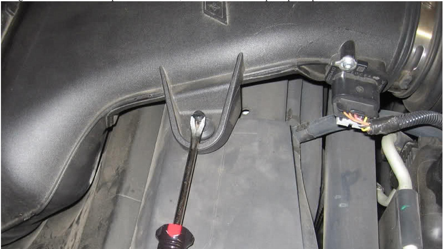
Figure 2. Remove the air intake retaining pins.
