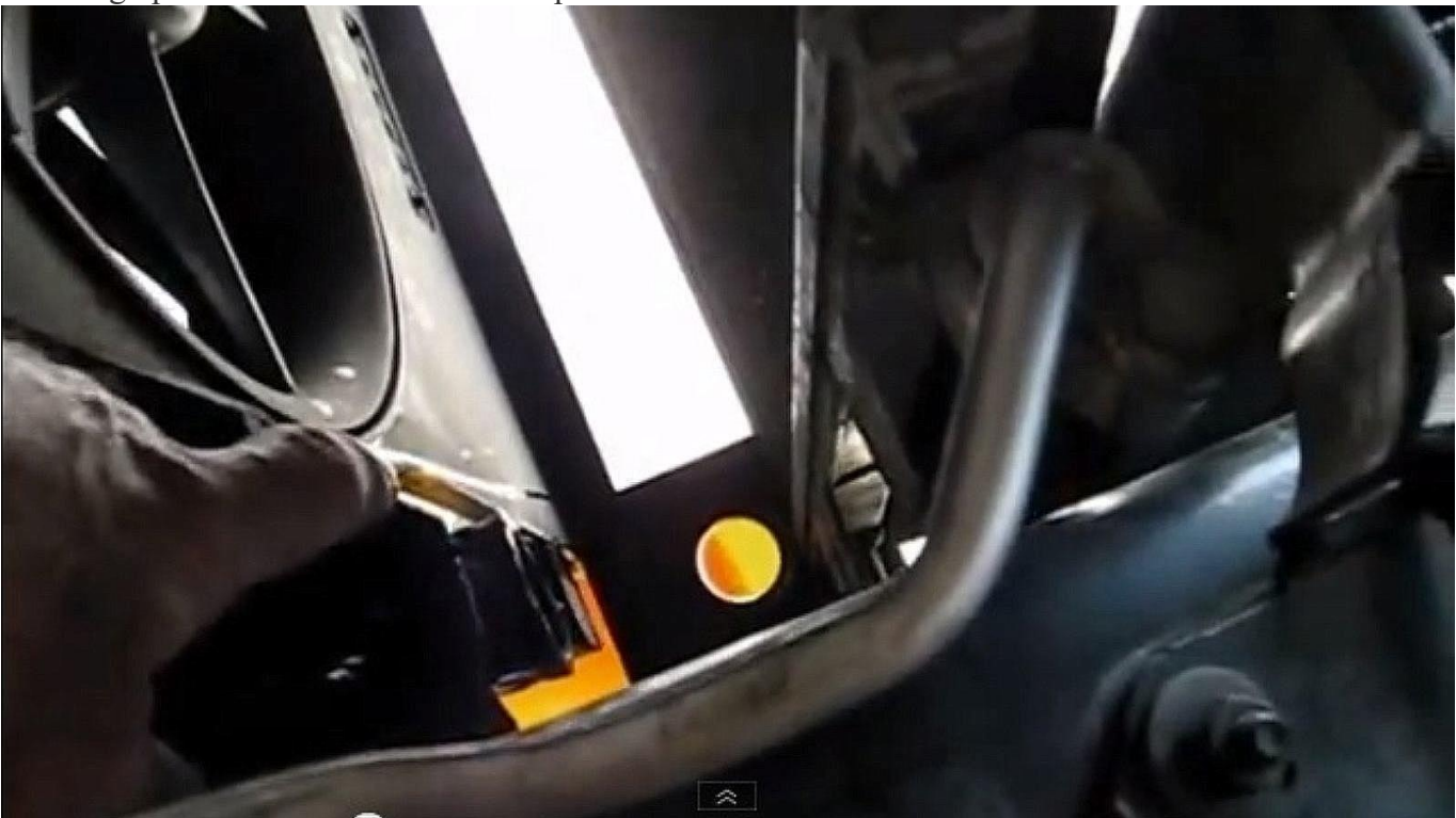
Figure 15. Electrical bundle on fan shroud that can hang up radiator extraction.
