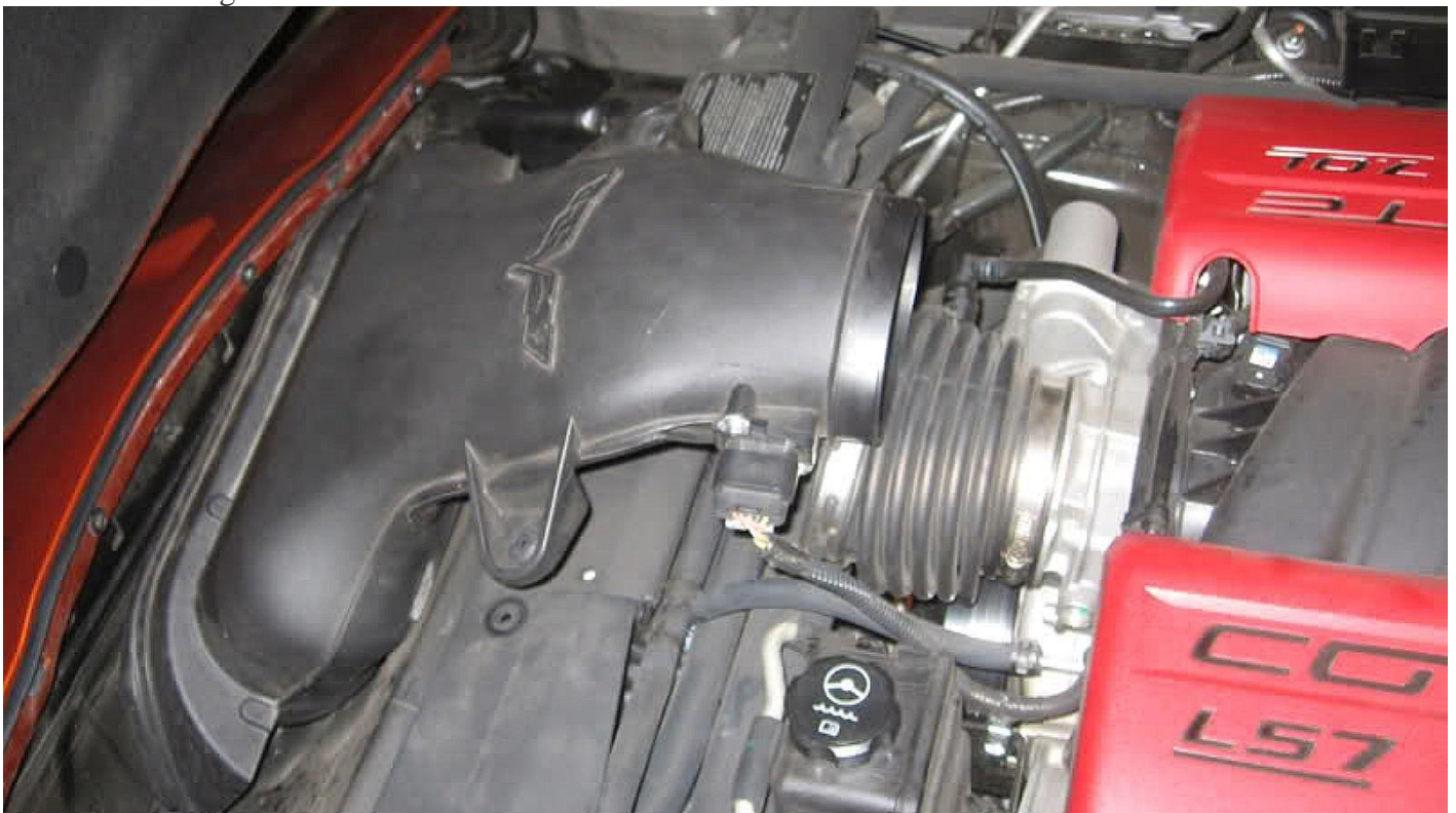
Figure 4. Disconnect the intake from the throttle body bellows.
