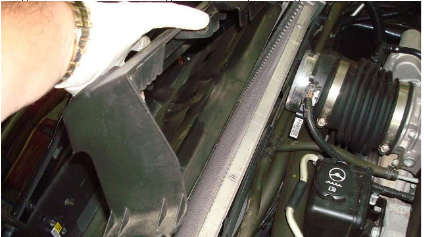
Figure 6. Remove the top radiator support.
