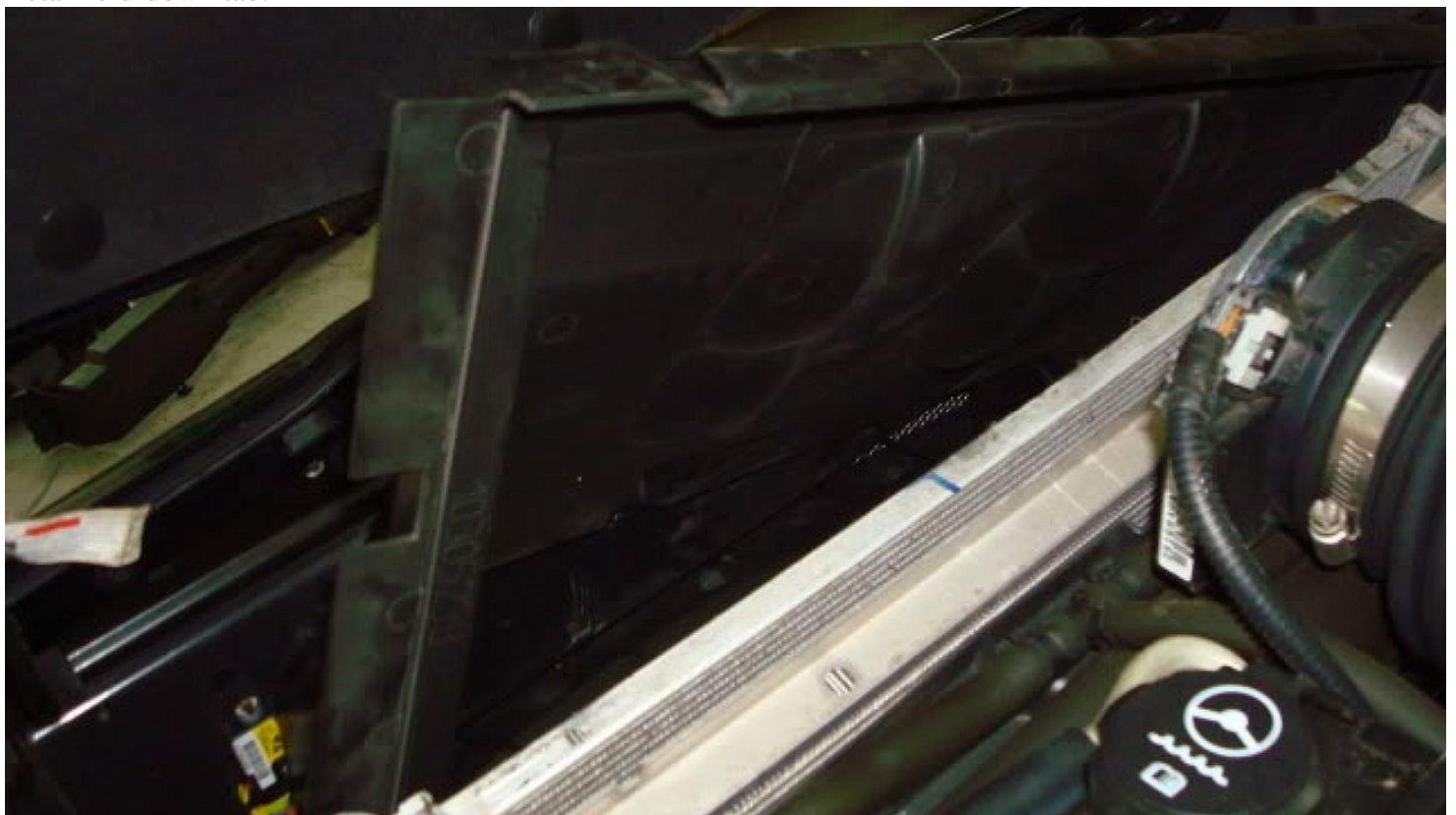
Figure 12. Tilt up and shove the shroud to free it from the other metal tab.
