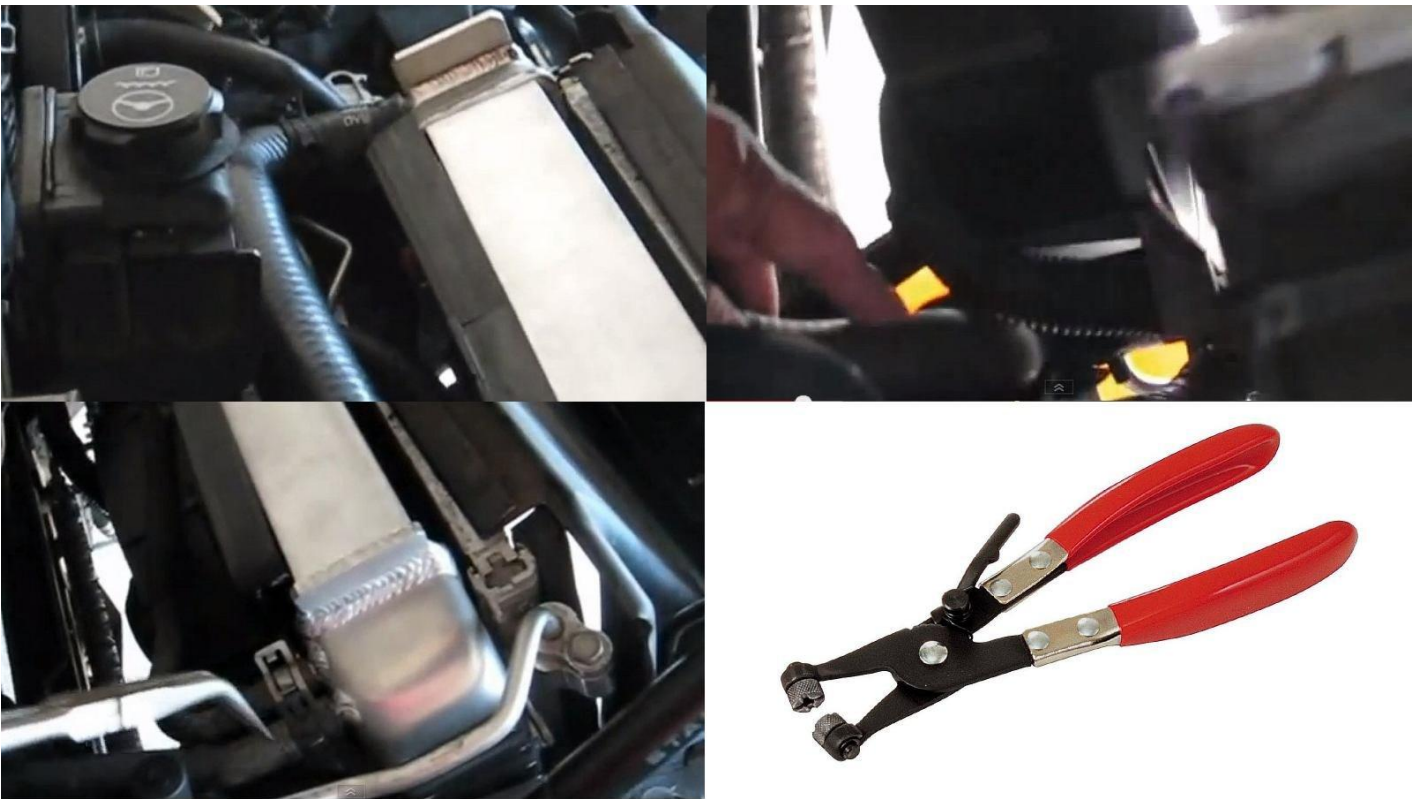
Figure 14. Remove the four hoses connected to the radiator with hose clamp pliers.
