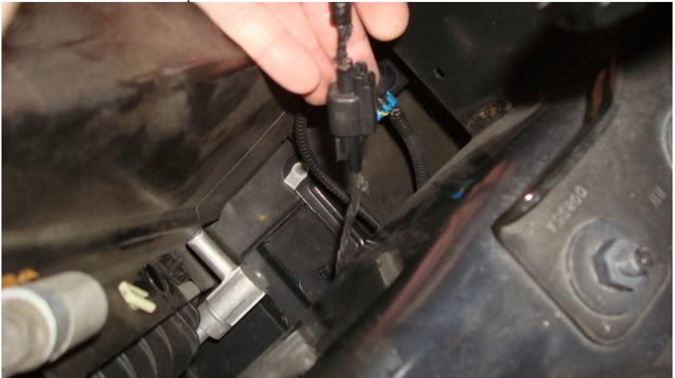
Figure 10. Disconnect the hood lamp connector, if you have one.
