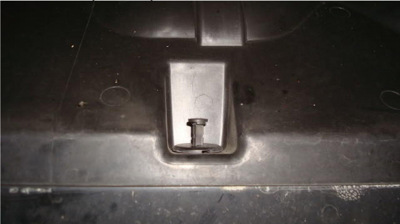
Figure 8. Remove pins that mount the bottom of the radiator shroud to the bumper beam.
