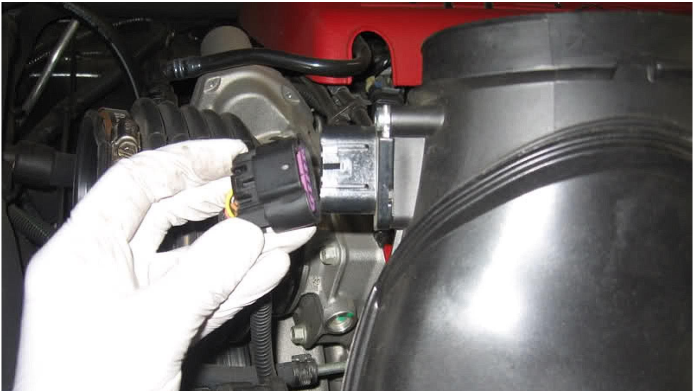
Figure 5. Unplug the MAF sensor harness.
