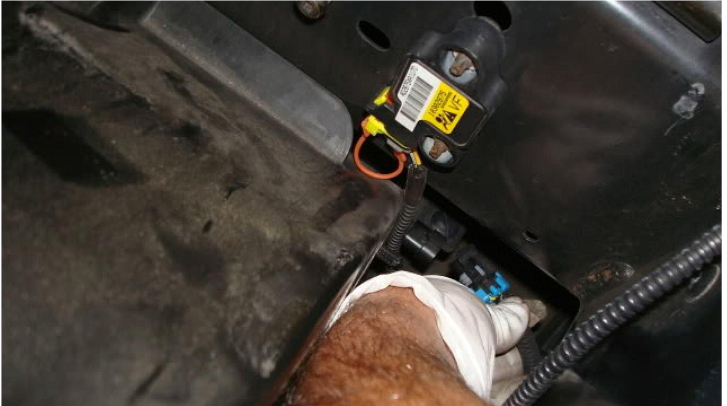
Figure 9. Disconnect the ambient air temperature sensor from shroud.
