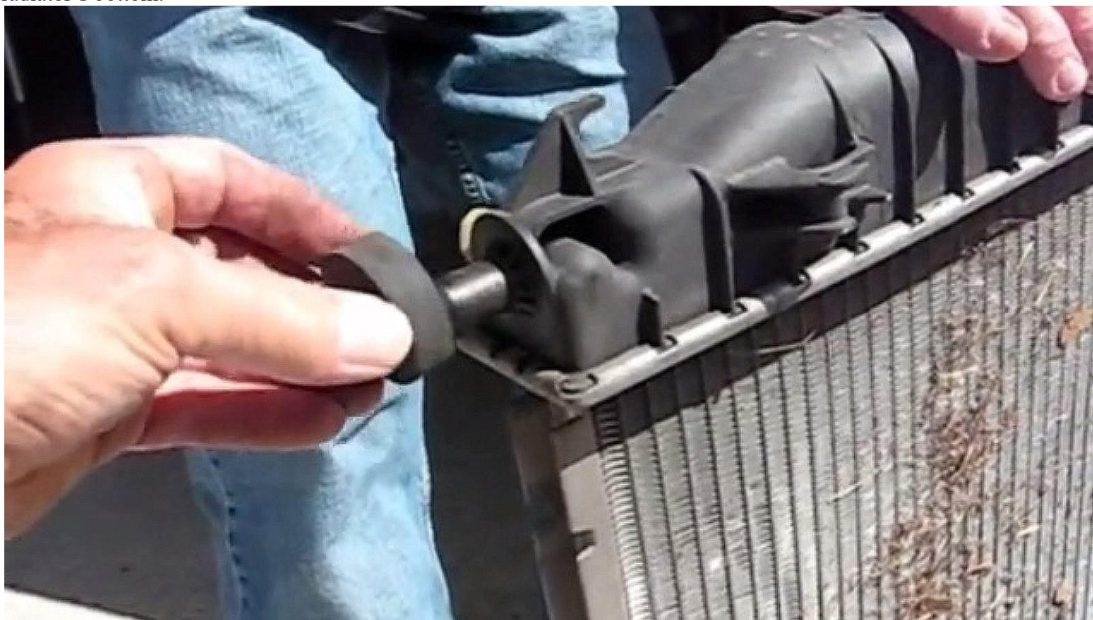
Figure 17. Rubber grommets act as "feet" and should be reused.
