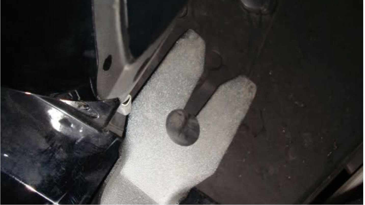
Figure 7. Remove push-pins mounted to the inside of the radiator shroud.
