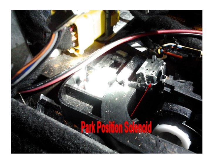
12) Assuming that your transmission is out of Park and stuck somewhere around Drive or Neutral. In order to release the Locking Pawl (tab), a small flat screwdriver can be inserted between the locking pawl and the catch, and pried up to get it released. Once this tab is released, then the shifter finger button can be pushed in, and easily moved into the Park position.
