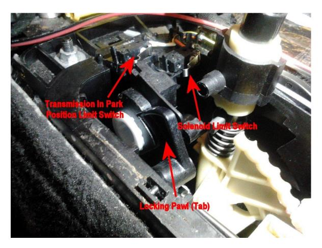
The above pics have: the shifter shaft (with black coupling), a solenoid contact limit switch in front of the shifter. This contact limit switch is made when the shifter is in Park. The contact has to be closed in order for the signal to be sent to energize the Transmission Lock Out Solenoid.
