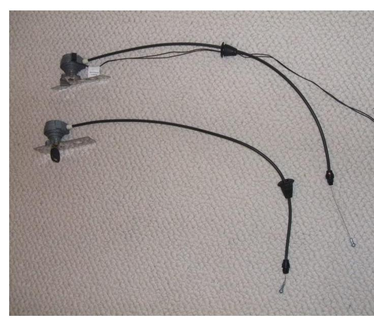
Also, you can just replace the inside of the lock cylinder (at least I guess you can buy just the inside piece). When I installed the auto pull down latch into my early Z06 I swapped that interior piece so that my one key would work the glove compartment/console/hatch:
