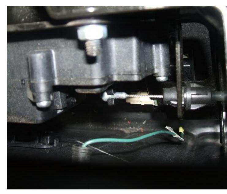
If the cable is not properly hooked into the latch release it will look like this:
