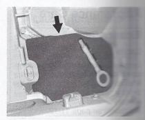
5. Remove the battery cover and locate the positive (+) and negative (-) terminals.
