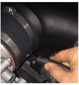
**Driver side 2014-2015 cars only:** Using supplied angle reducer hose, short PCV line and angle cut barb Assemble by sliding the 3/8ths hose INTO the angle reducer hose (no clamp needed here) now place the barb into the 3/8ths hose with the angle cut facing the throttle body for clean pull of vacuum.
