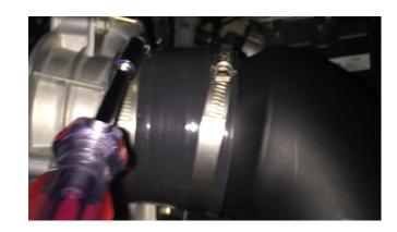
This will pull the Joint between the Air-box tail and intake tube in opposite directions and <u>SET</u> the intake tube and Air-box joint angle (as shown below)
