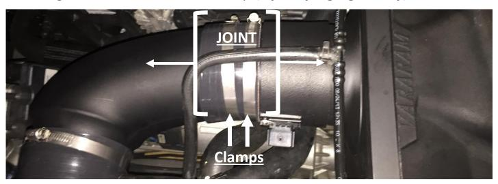
A quick double check step to check your work - Remove the system as one unit ,leaving JOINT hose clamps tight. Once removed run your arm in from the throttle body side and FEEL for the transition at the Air-Box tail to intake tube connection (as shown) feel for any gaps on the short-side radius , if so slide the intake tube clamp down further and retighten.
