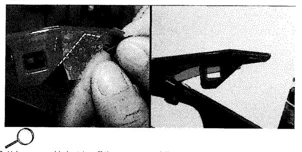
12.3. Using a razor blade, trim off the excess tape following the molded contour of the fascia.
