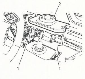
2. Remove the upper closeout boot (2) from the transmission control assembly.
