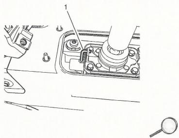
10. Lift to release the shift control neutral lock pin (1).
