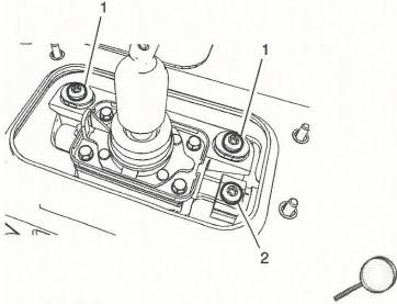
9.6. Tighten the shift control mounting bolts (1) to 30N·m (22 lb ft).
