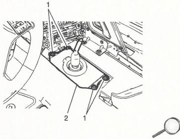
11. Install the lower transmission control closeout boot (2).
