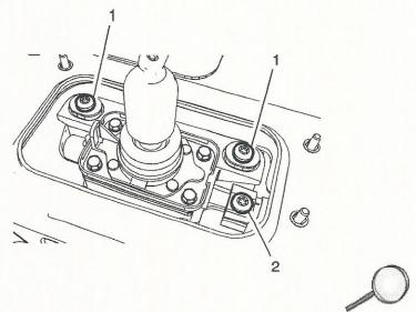
9.4. Inspect for proper alignment in the Neutral position.
