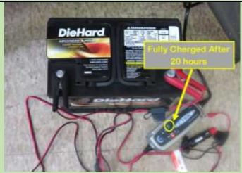
Used my CTEK 3300 to fully charge the battery before installing. In < 20 hrs it showed fully charged.
