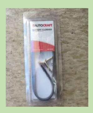
There is no way to grab the battery to lift it out of the well. You'll need a tool! I bought this inexpensive one locally. It connects to the battery terminals. It worked OK but the terminals are on one side of the battery so it tilts. It also slipped off once when I started to lift!
