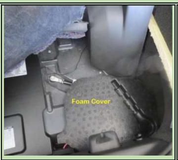
A hard foam cover just sits on top of the battery. That is what is between whatever is put in on the hatch floor and the top of the battery. It must fit properly.
