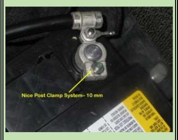
The first thing to disconnect from a safety standpoint is always the negative battery cable terminal. The C7 uses a positive mechanical clamping mechanism. No need to spread terminals, just loosen the 10-mm nut and the terminal slips easily off the battery post.
