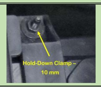
Now the two 10 mm nuts that fasten the plastic hold-down are removed. Be careful not to drop them, however no big deal now as when the battery is removed you'll find them in the battery well!
