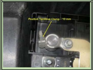
The positive terminal clamp is similar to the negative terminal. It is a mechanical fastening device, no spreading of a clamp required. Also, no need to remove any other nuts as the whole fuse block assembly will be moved as a unit. I just tuned it upside down and moved it to the left of the battery well on to the hatch floor.
