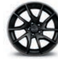
19" x 10" Front and 20" x 12" Rear Z06 10-Spoke Blade Machined-Groove Aluminum Wheel in Black 2
