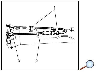
21. Disconnect the inline connector of the clutch pipe (2) then disconnect the clutch line retainers (1) from the driveline support tube and secure the body side of the line aside (up).
