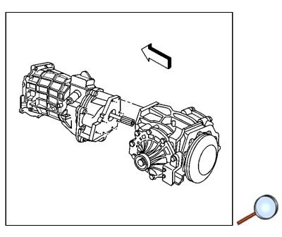
42. Remove the differential to transmission bolts and nuts.
