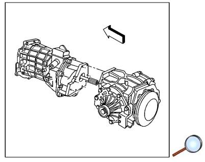
4. Install the transmission to the *J*-42055 transmission support fixture , if removed.
