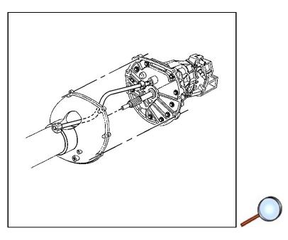
39. Slowly slide the driveline support assembly away from the transmission while guiding the transmission shift rod through the opening in the driveline support assembly.
