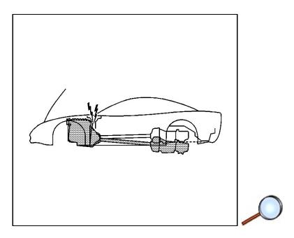
**Caution:** When tilting down the rear of the driveline, observe the clearance between the rear of the engine and the composite dash panel. Do not allow the engine to rest unsupported against the composite dash panel, or vehicle damage may result.
