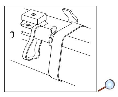
12. Loosely install a rubber band onto the transmission shift rod and position just behind the shift rod clamp.
