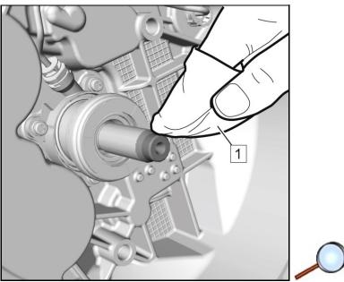
**Caution:** Ensure that no grease remains on the lead surface of the transmission input shaft. Clean the lead surface of the transmission input shaft prior to the assembly of the transmission to the engine. Failure to maintain a clean surface may cause clutch slippage or failure. 3. Clean the entire lead surface of the input shaft with a NEW, lint-free towel (1).
