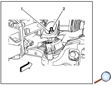
**Note:** Hold the transmission mount stud (2) with a suitable wrench to prevent the stud from rotating in the mount. If the stud becomes loose, replace the transmission mount.
