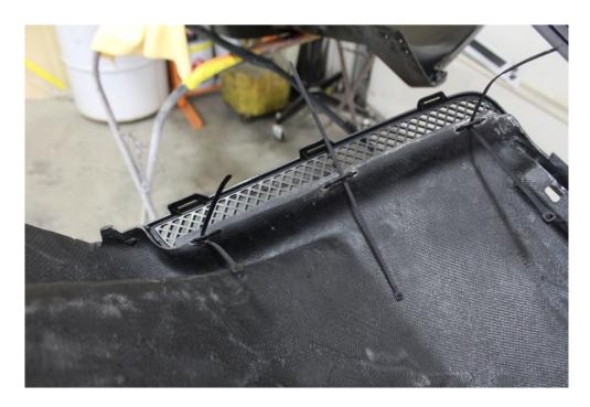
Bolts behind the reflectors - before you put the reflectors back into the diffuser and before you put the bolts in to attach the upper and lower bumper together, you will put the metal brackets into the lower diffuser to to add stability when you tighten the bolts down. Make sure these go on the OUTSIDE of the diffuser, not between the upper and lower bumper inside. Basically, they'll push the reflectors only out slightly.
