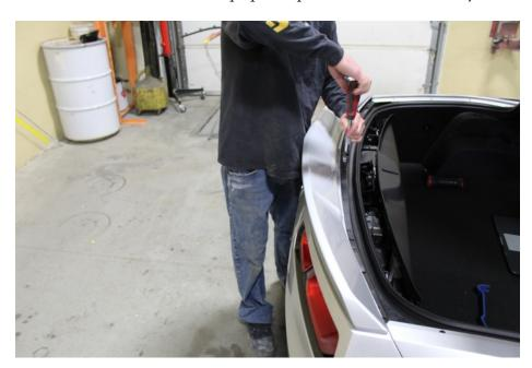
in by clips so start at one end and work your way to the other and it pops straight out to reveal the T15 Torx screws that need to be removed.
