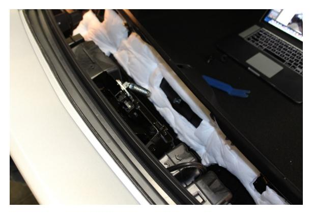
Step 3: Now you can remove the tail light bezels. Using a tool with a hook on the end helps to pull the mesh between the louvers in one corner. It's pretty resilient and just held in by clips, so apply pressure till it pops out and then slowly work your way around the lights removing one clip at a time. This will allow you to remove the two T15 torx screws on the upper inner tail light areas. A flashlight might be needed to see them.
