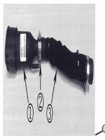
**Note:** Take care when removing the filler hose not to damage the filler pipe seal bead or corrosion resistant paint.
