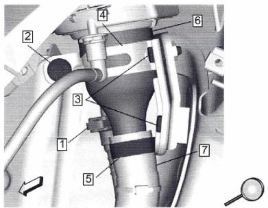
2. Remove the fuel tank filler pipe (6) from the vehicle. Refer to *Fuel Tank Filler Pipe Replacement* in SI.
