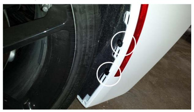
Exercise Caution! Use hook end driver and hook the tool in the mesh part of the bezel around your taillights. Pulling back, the corner will release. Once the corner is released you will be able to persuade the rest of the bezel out. Repeat step for the other side.
