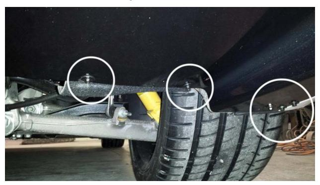
Remove the mud flaps; these are just snapped into the bumper. Recommended to use a plastic pry tool to get started; once started you can pull the rest by hand. After the mud flap is removed, it will reveal two T15 Torx screws. Remove these as well.
