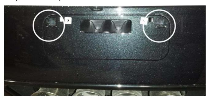
Remove 10mm bolts located just above the exhaust tip. Recommended use of 6-inch extension for these.
