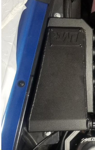
Figure 3 Both bolts installed and breather aligned
