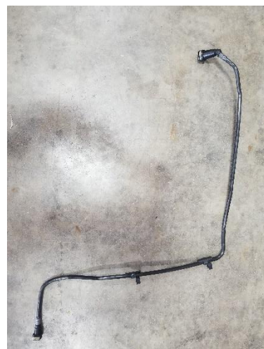
Figure 5 PCV line to remove from Driver side valve cover
