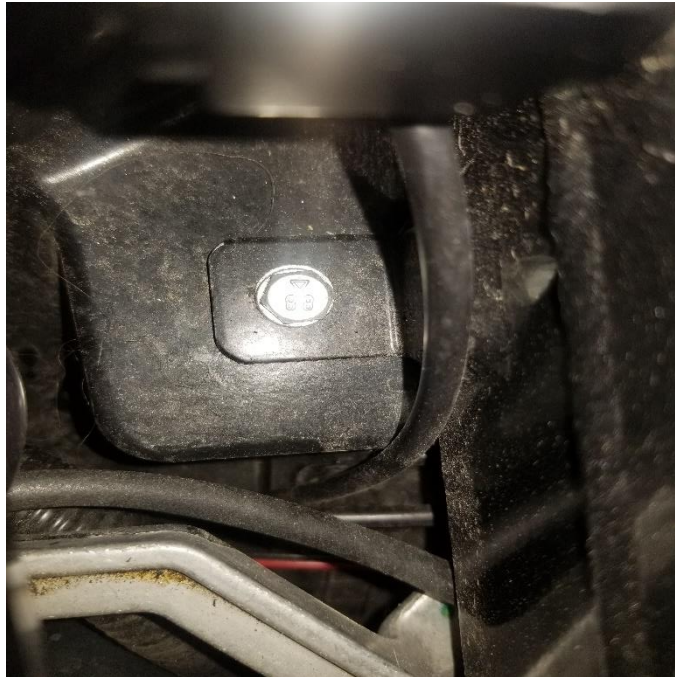
Figure 2 Slide bolt through Retainer clip hole
