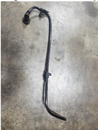
Figure 4 PCV line to remove. Cut quick disconnect from end that connects to dry sump
