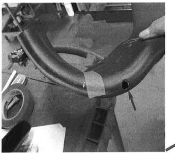
5. Measure 50.8 mm (2 in) up from the hole. Mark and cut using a hack saw.
