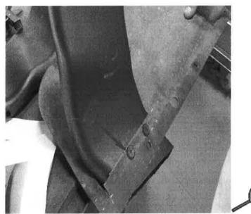
6. Place the cut duct into the slot. Make sure it comes out of the slot 25.4 mm (1 in). Using a 1/4" drill bit, drill 2 holes through the deflector and duct and rivet together.
