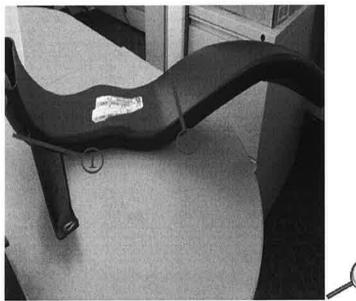
4. Using a hack saw, cut the support arm off (1) and the duct after measuring 50.8 mm (2 in) (2) after the second bend.
