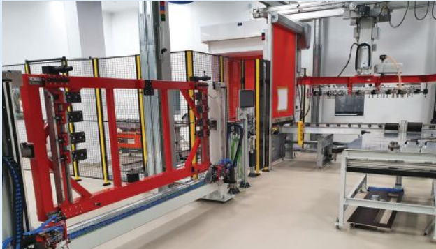
7 Preformed spar kits are next assembled around mandrels that are loaded into a cassette (red frame on left) prior to placement in the mold.
