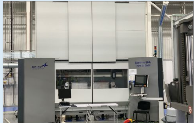
11 Molded spoilers are loaded into one of two CMS CNC machines for trimming and drilling.
