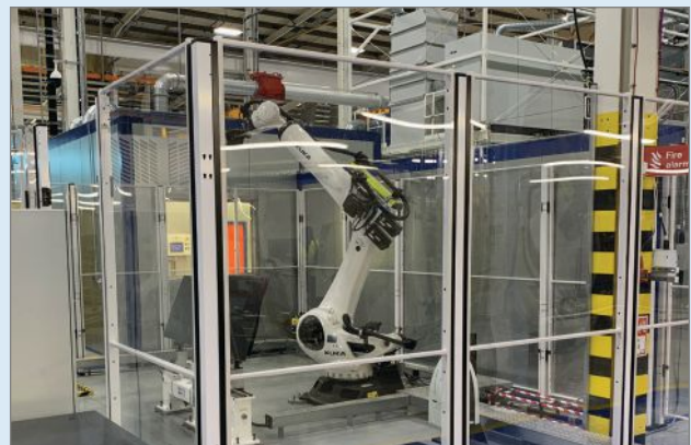
12 Following machining and prior to final assembly of metallic fasteners, each spoiler is inspected using multiaxis robots and phased array UT systems.
