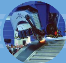
Automated Fiber Placement Gantry
