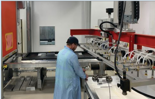
8 An operator stands at a workbench before the lower half of an A320 spoiler RTM mold, prior to lower skin, spars and upper skin preform loading. Each spoiler variation has three aluminum molds.
