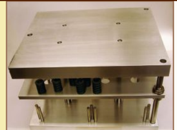
ASTM C297 SANDWICH PANEL FLATWISE TENSILE BONDING FIXTURE
