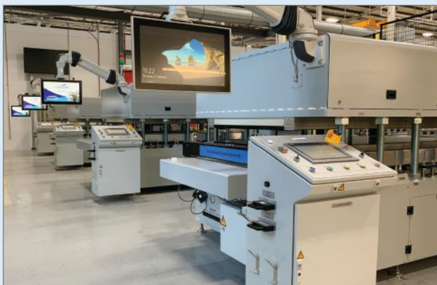
9 After the top half of the spoiler mold is secured to the bottom half, the entire tool is transferred to one of seven Coexpair RTM presses that Spirit has installed. The resin injected is Hexcel's RTM6 single-component epoxy.
