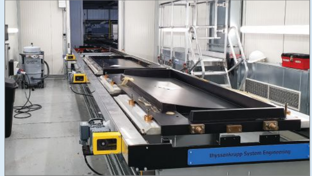
10 Following molding, finished spoilers are demolded. Tools and mandrels — loaded vertically on a carousel — are then cleaned and conditioned before returning to the production line.
