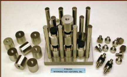
ASTM D7291 LAMINATE TENSILE THRU-THICKNESS BONDING FIXTURE
