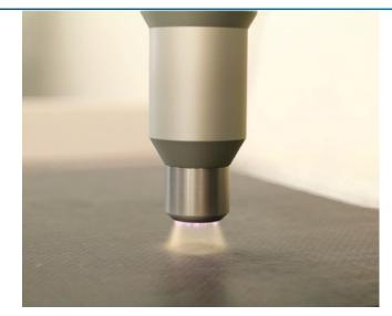
When optimized and verified through reliable testing, plasma is an effective way to change the chemical composition of the surface of a material that is to be bonded. Source, all images | BTG Labs
