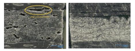
Laminate using wet winding with voids (left) compared to a near void-free laminate created with towpreg (right). Source | TCR
