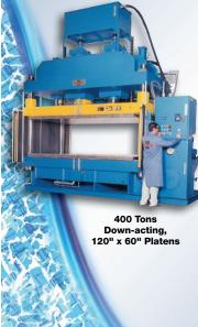
produces a wide range of hydraulic presses for compression molding in composites applications. We offer standard and custom designs from 15-1000 tons with various heated platen sizes and control options. Visit our website to learn more.
