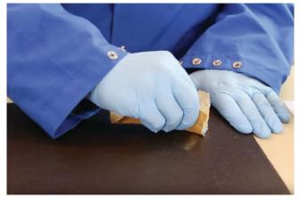
Manual abrasion is a common method of surface preparation for composites, but it may not be effective at cleaning a surface on its own.
