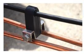
3D-printed PLA clips serve as intermediate droppers, attaching the CF/TP epoxy catenary 70-mm above the copper contact wire
