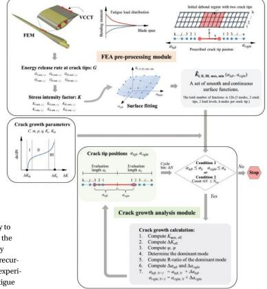
**FIG. 1** Flow chart of the proposed FASTIGUE approach comprising an FEA pre-processing module (top) and a crack growth analysis module (bottom). Gray arrows indicate the computational flow, showing that feedback between the FEA pre-processing module and the crack growth analysis module is avoided, resolving heavy computational demands of fatigue crack simulation for large structures such as composite wind turbine blades. Source | Martin Eder, Xiao Chen, DTU Risø
