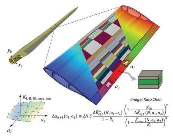
**FIG. 2** In FASTIGUE, an initial through-crack is introduced at an arbitrary location along the bondline of a 3D finite element wind blade model. The crack proceeds away from this point in both directions along the bondline at the blade's trailing edge. The fracture parameters (e.g., the stress intensity factor, *K*) can be computed in both crack tips for a number of user-defined crack lengths on both sides denoted as <sub>aland a2</sub>. Source | Martin Eder, Xiao Chen, DTU Risø
