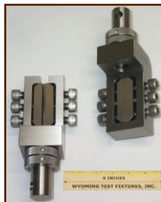
V-Notched Rail Shear Test Fixture ASTM D 7078
