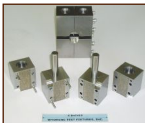
Combined Loading Compression Test Fixture ASTM D 6641
