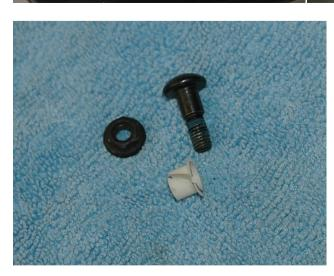
3. With the headlight tilted down, remove the 10mm nut that holds the headlight lifting arm to the headlight motor. Disconnect the headlight bulb sockets and remove the headlight (picture shows the placement of the nut without the headlight.
