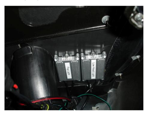
c - You can also make a VERY secure, yet easily removable mount by drilling through the wheel well wall and bolting the ballast directly to the wall.
