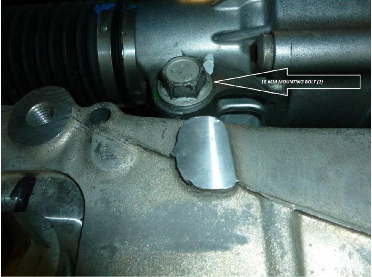
LEFT SIDE STEERING RACK MOUNTING BOLT
