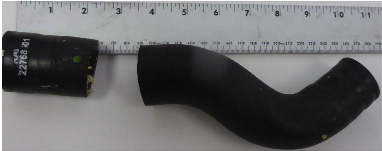
SECTIONS REMOVED FROM RADIATOR HOSE
