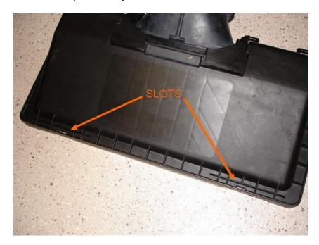
Mark and create holes for straps directly beneath the clips.
