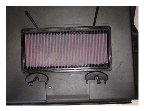
Install air box by sliding the ties through the slots at the bottom of the airbox securing with the ends cut from two Zip Ties.
