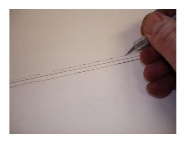
Remove the paper from the radiator shroud, and using the holes previously made in the shroud as a guide, score the plastic with a razor knife against a straightedge. Then follow the scored line with straight cutters.
